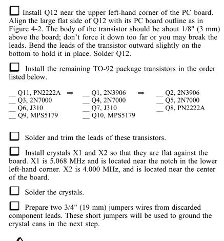
Grounding the crystal cans in the following step is required to ensure proper crystal oscillator performance.
