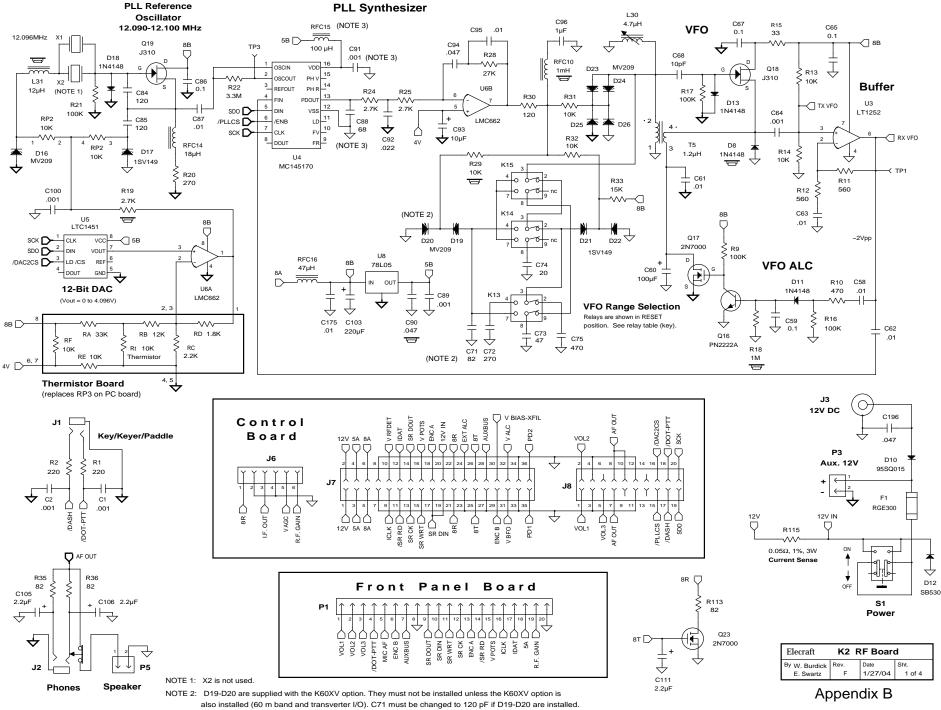
NOTE 3: These components improve PLL stability; they must be soldered on the back of the board (see text).
