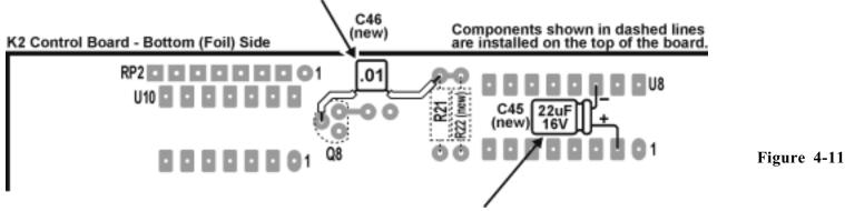
A 22-µF electrolytic capacitor has also been added (C45). Solder C45 as indicated above, between U8 pin 2 (+ lead) and U8 pin 14 (- lead).
